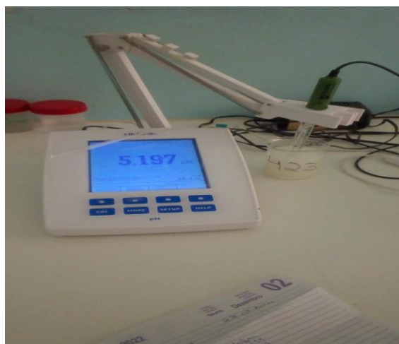
Figura E-1. pH metro (HI 1131 da HANNA Instruments)
