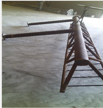
Picture before abrasive blasting
