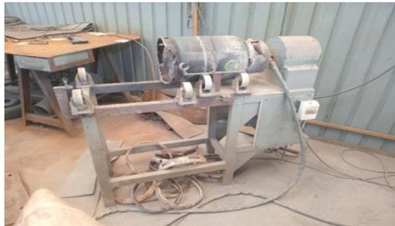
Figura 13: Corte a plasma manual
