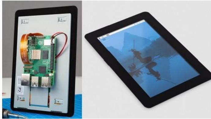
Figura 2.12: Raspberry Pi Touch Display 2. Fonte: [RaspberryPiTouchDisplay2024]
