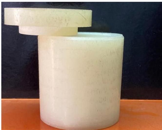
**Figura 11** – Vaso interno do reactor.
