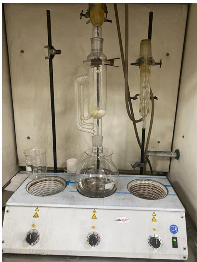
Figura A7-4: Extractor de Soxhlet.
